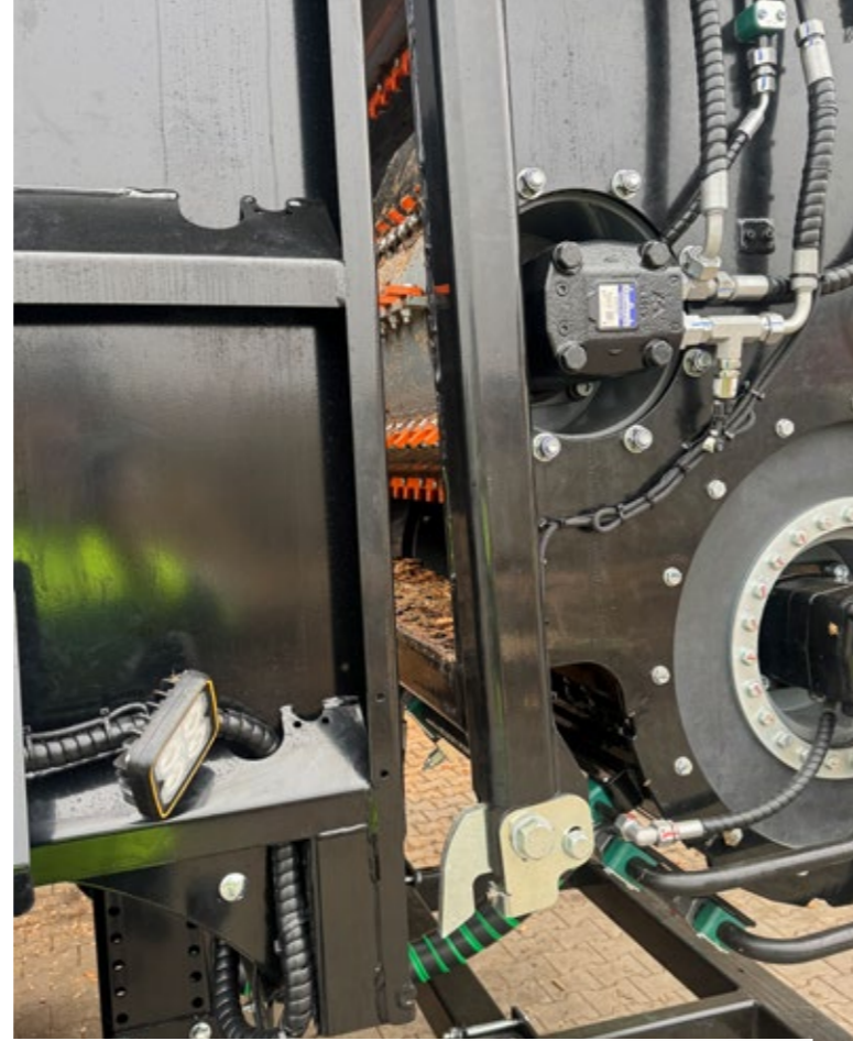
Rear flap can be opened for maintenance
